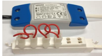
NOTE: FITTINGS ARE WIRED IN SERIES
