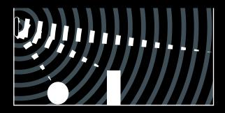
When a moving object enters the area the sensor receives a new reflection, which trips the sensor and turns on the light.
