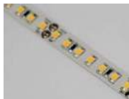
LED strip Linear 140 140 led | 14 W | 1540lm
