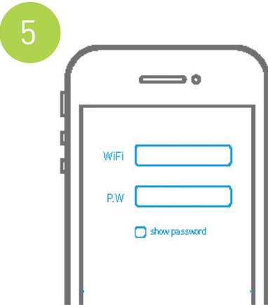
5 Enter your own local Wi-Fi name and password. Then click on the configuration/setting button. It will automatically configure and may take within 30 seconds to complete.
