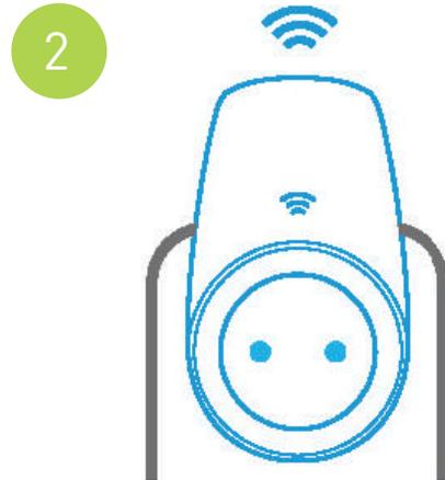
2 Plug the SMART Wi-Fi Box into a power outlet and switch ON. The Wi-Fi indicator light will light up red. The Wi-Fi Box is now ready for synchronisation.
